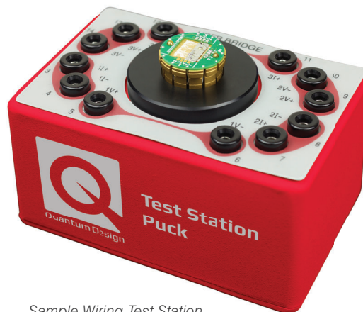
Sample Wiring Test Station
